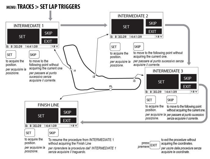
Every time the **SET** button is pressed the Best LED will flash white (to confirm the button has been pressed) immediately followed by a Green flash if the coordinates are correct or Red if GPS signal was missing.
