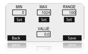
Since the throttle opening is expressed as a percentage by using values between 0% and 100%, the RANGE shall be set to 100.
