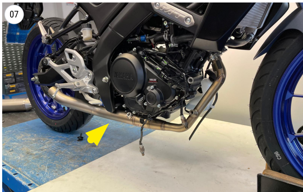
fit the pipe
