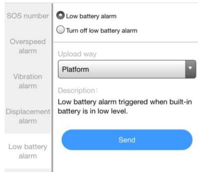
**Low battery alarm (only GPSANGEL 20):** when vehicle battery voltage quando la batteria del veicolo drops below 11 V , GPSANGEL sends an alarm and remains active using its internal battery.
