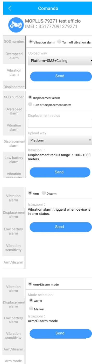
It's the movement-detection alarm. When the vehicle is moved with engine OFF, GPSANGEL sends an alarm notification.
