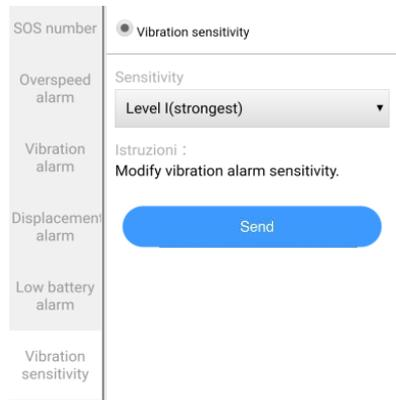
**Vibration sensitivity:** it's the movement-detection sensitivity setting (only GPSANGEL20). Level1 most sensitive, level5 is less sensitive.
