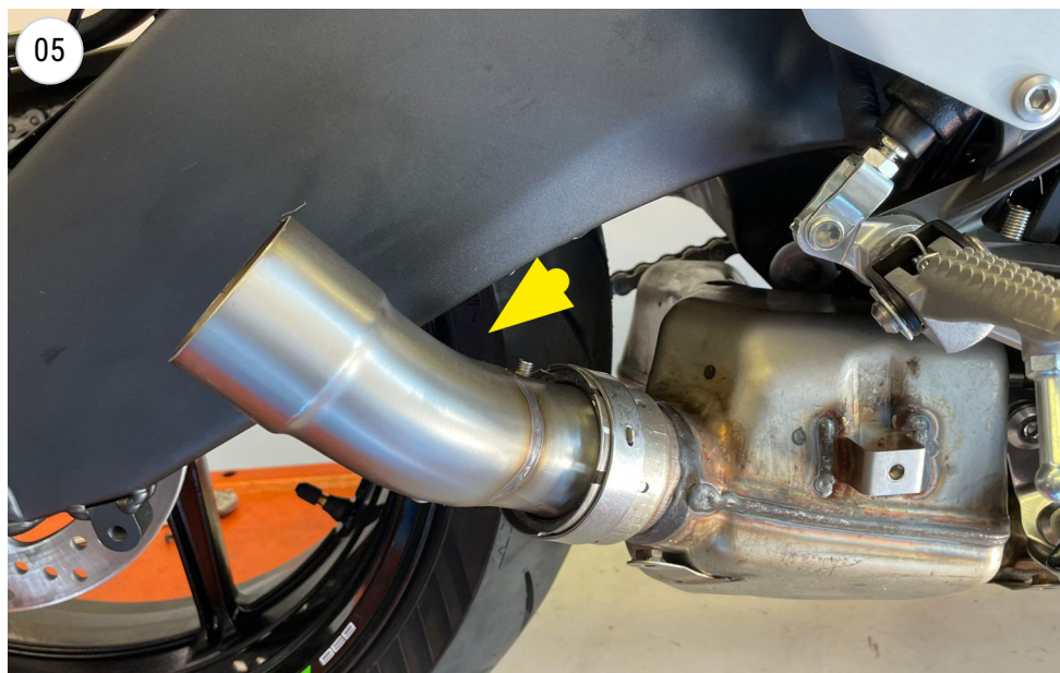
fit the pipe
