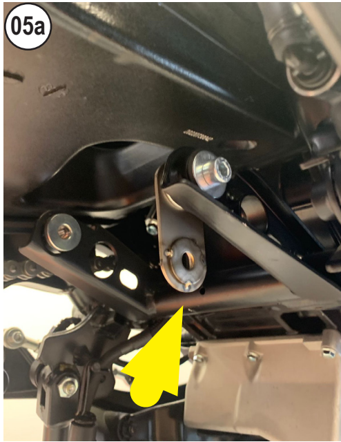
INSTALL THE BRACKET
