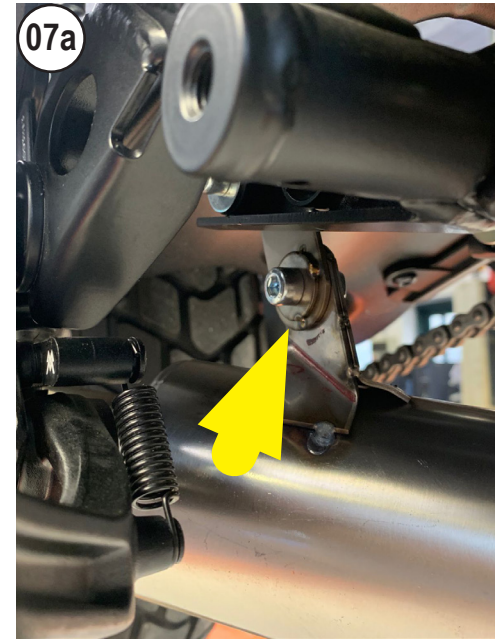
FIX THE PIPE AT THE BRACKET
