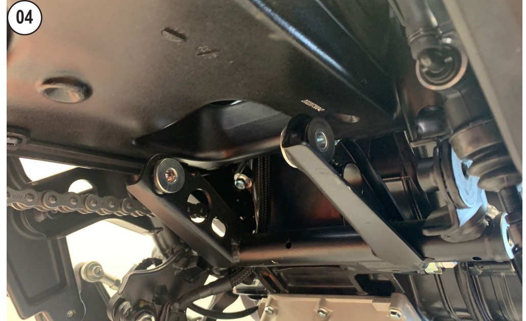
REMOVE THE STOCK MUFFLER
