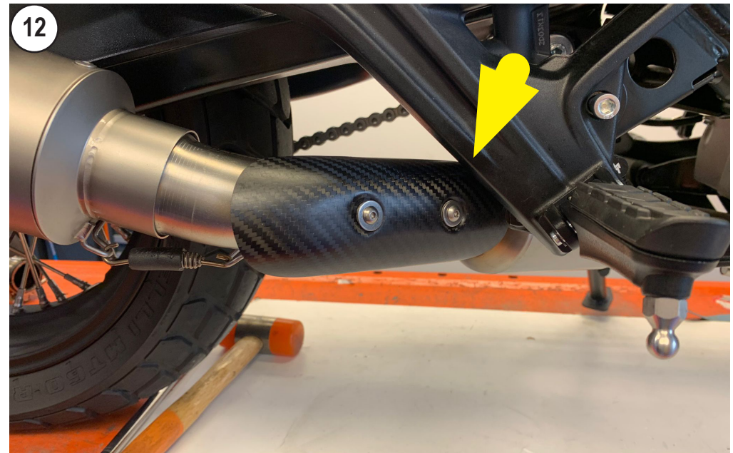
INSTALL THE CARBON HEAT SHIELD
