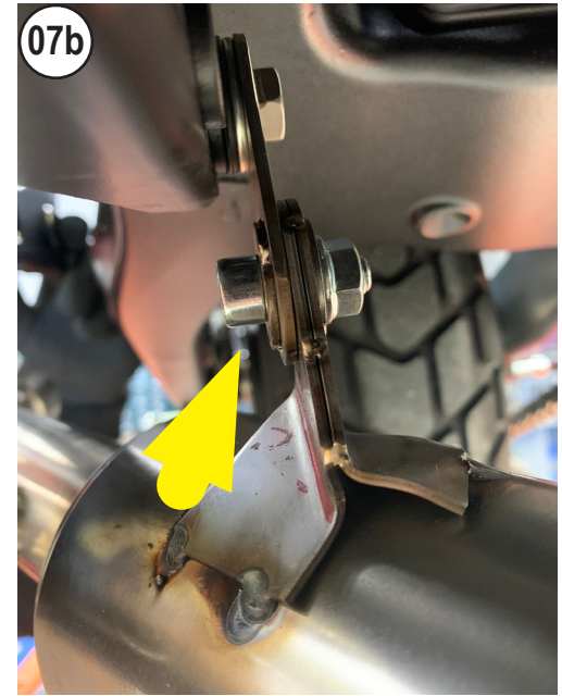
FIX THE PIPE AT THE BRACKET
