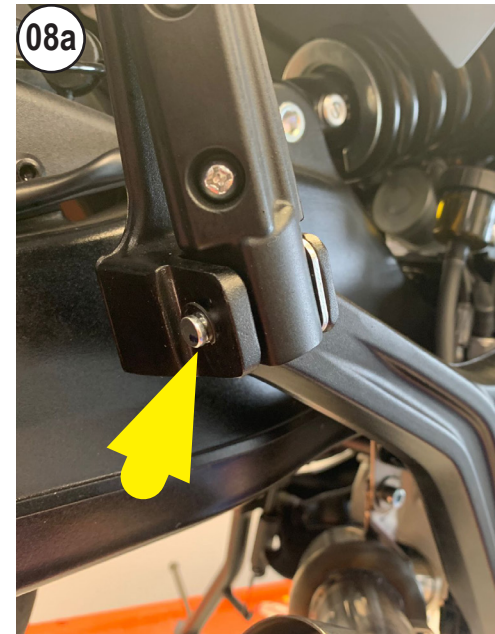
REMOVE THE SEEGER AND THE PIN
