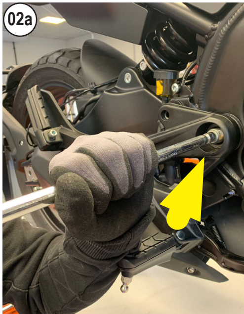
TAPPING THE PIN TO BRING IT BACK
