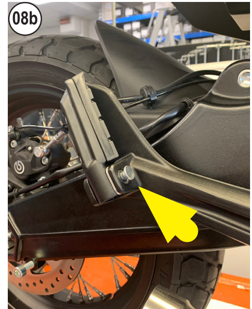
REMOVE THE SEEGER AND THE PIN
