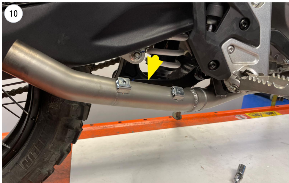
fit the final pipe
