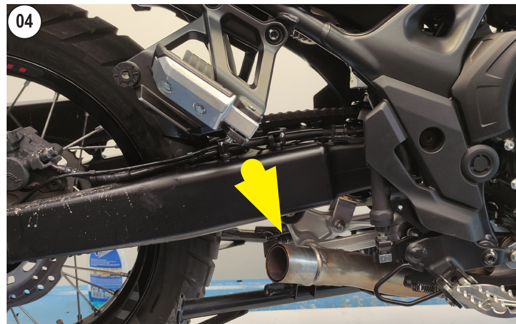
REMOVE THE ORIGINAL MUFFLER
