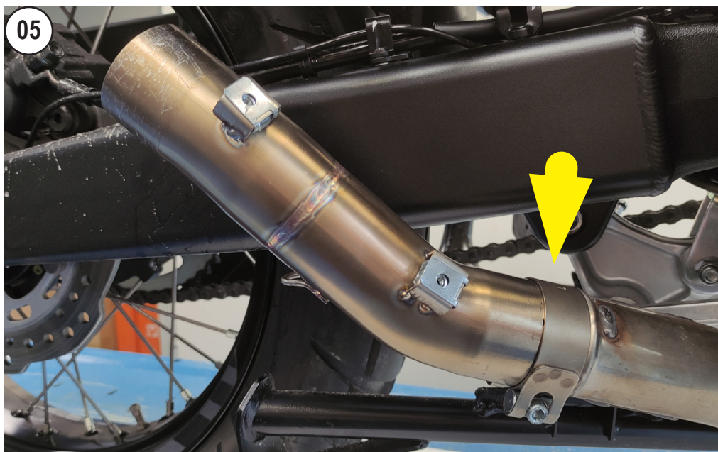
SLIDE THE PIPE IN WITH THE CLAMP
