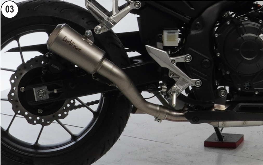
CORRECT ASSEMBLY - HONDA NX 500
