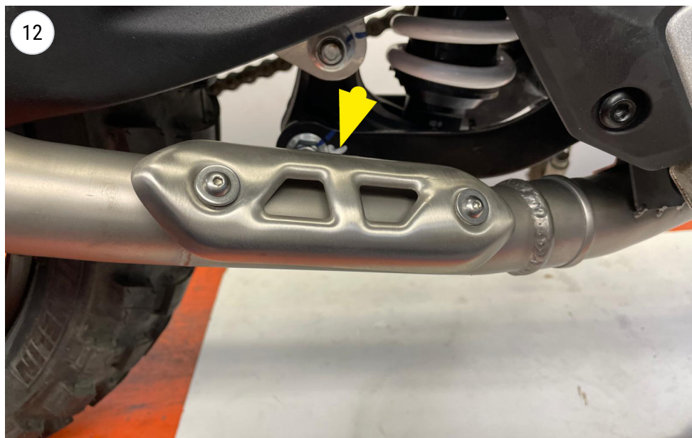
install the heat shield
