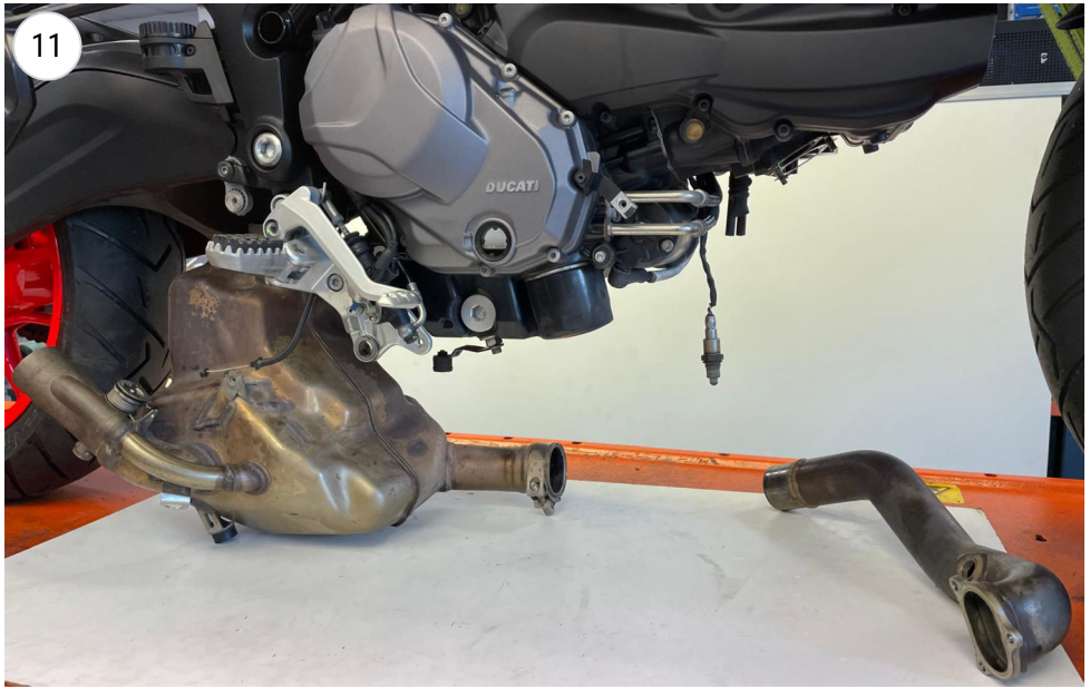
Remove the entire stock exhaust
