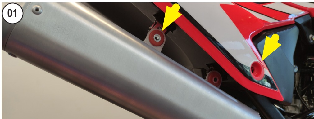
UNSCREW AND REMOVE THE STOCK MUFFLER
