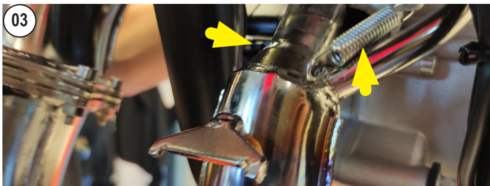
REMOVE THE SPRING AND REMOVE THE STOCK MUFFLER
