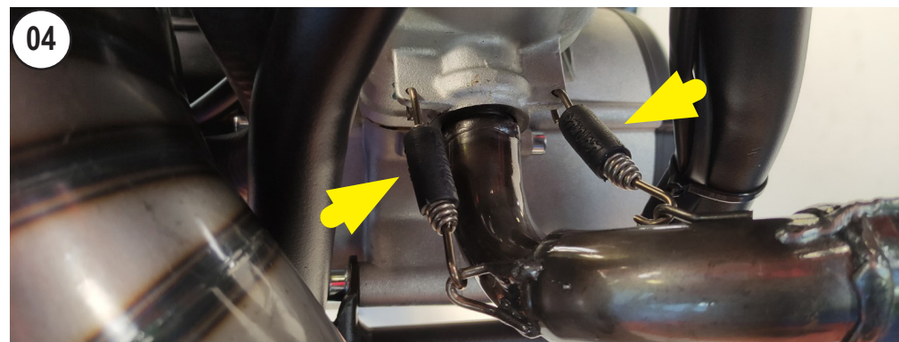
FIT THE LeoVince's HEADER PIPE AND HANG THE SPRINGS
