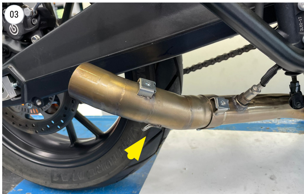
install the pipe
