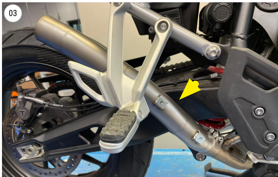
fit the pipe
