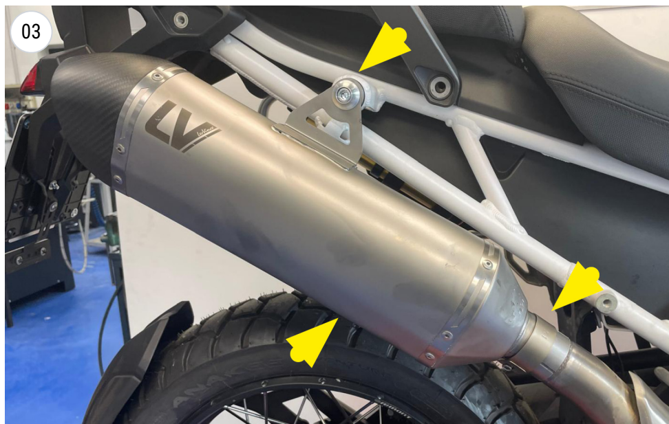
install the muffler with the clamp
