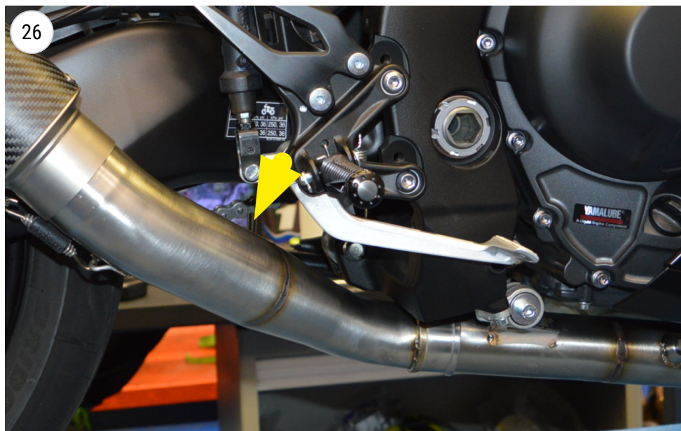
fit the final pipe
