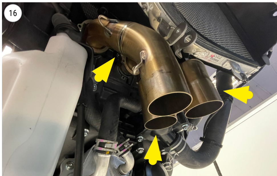
fit the primary pipe
