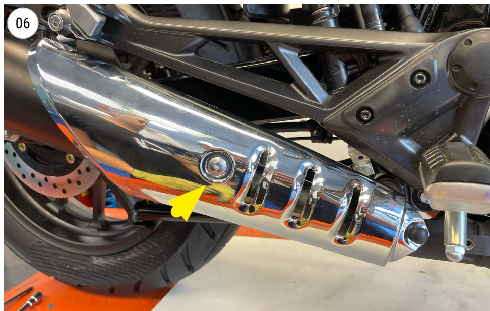
re-install the stock heat shield
