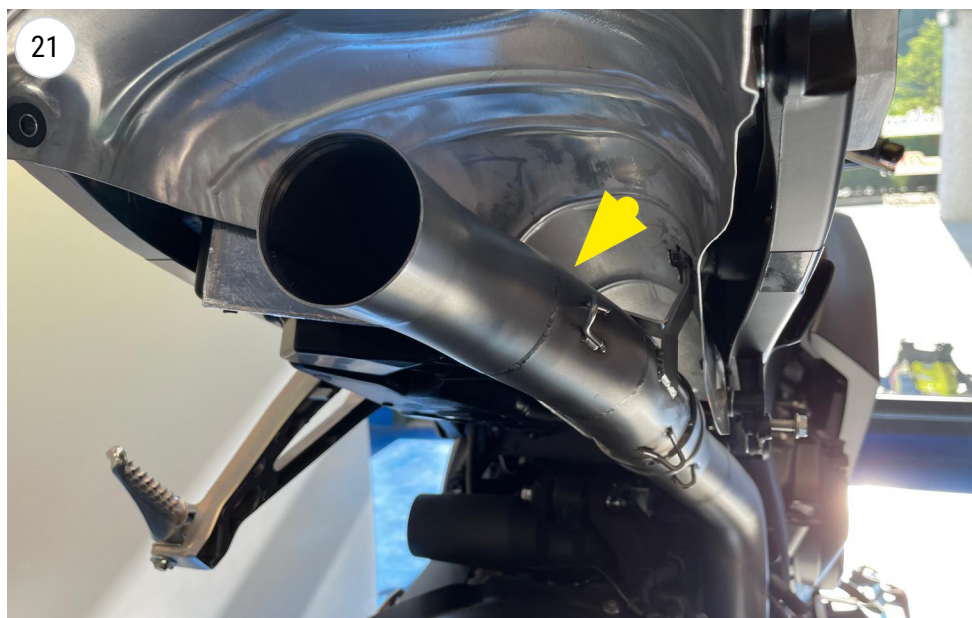
fit the final pipe
