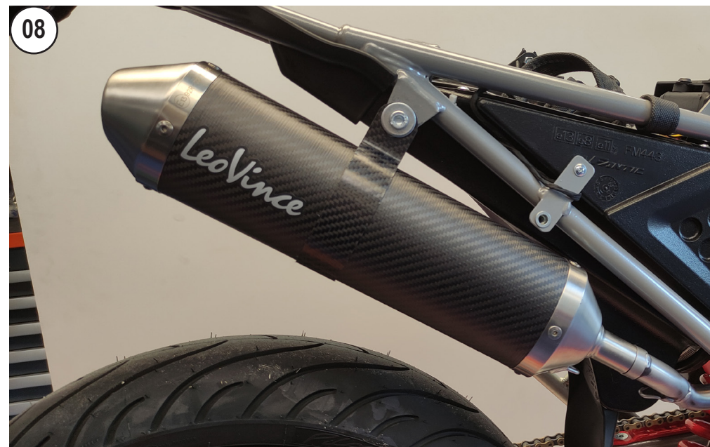
08 INSTALL THE MUFFLER
