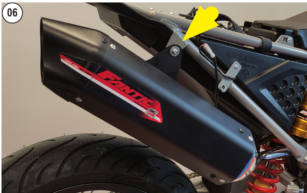
06 UNSCREW AND REMOVE THE MUFFLER
