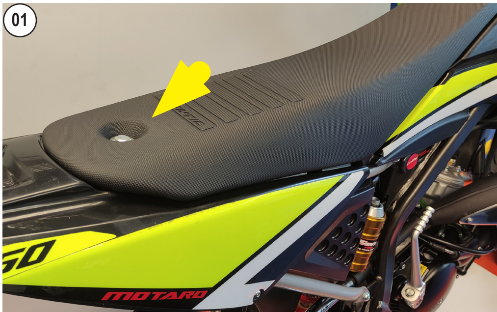
UNSCREW AND REMOVE THE DRIVER SEAT
