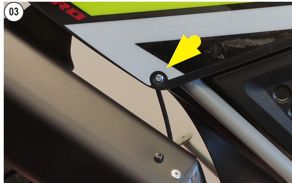
UNSCREW AND REMOVE THE SIDE PANEL
