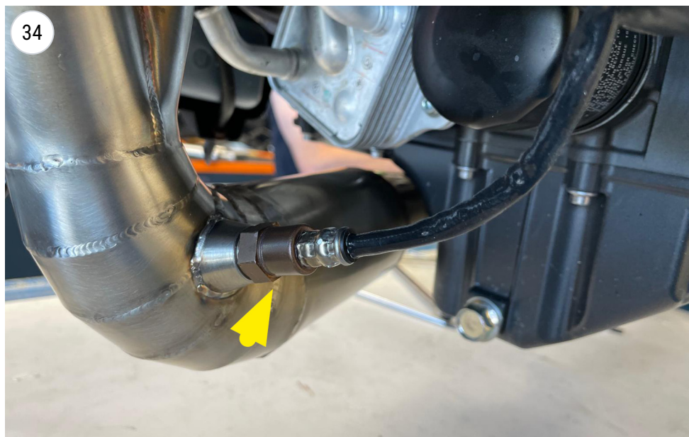
screw the sonda lamba / O2 sensor
