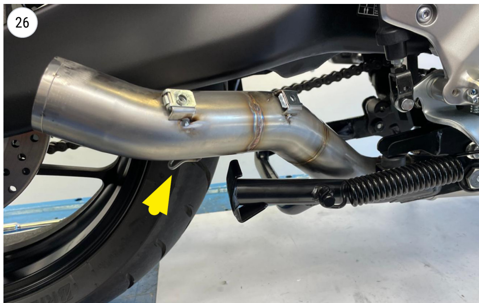
fit the final pipe
