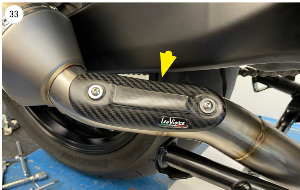
install the carbon heat shield
