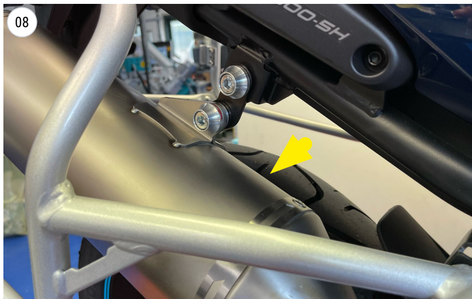
install the muffler (CF MOTO MT 800)
