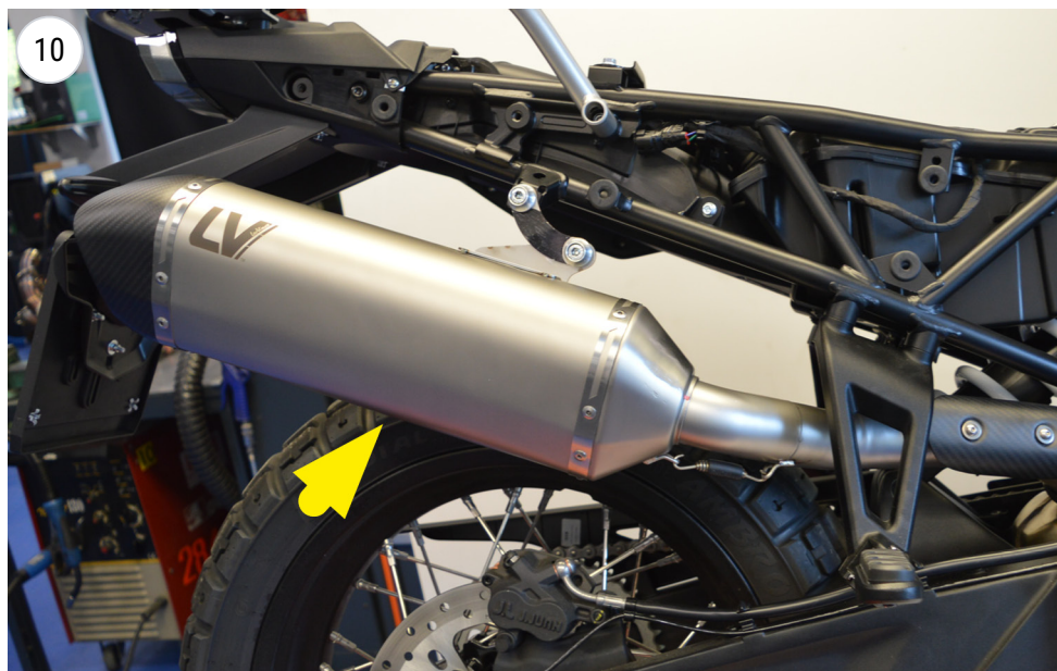
install the muffler (CF MOTO MT-X 800)
