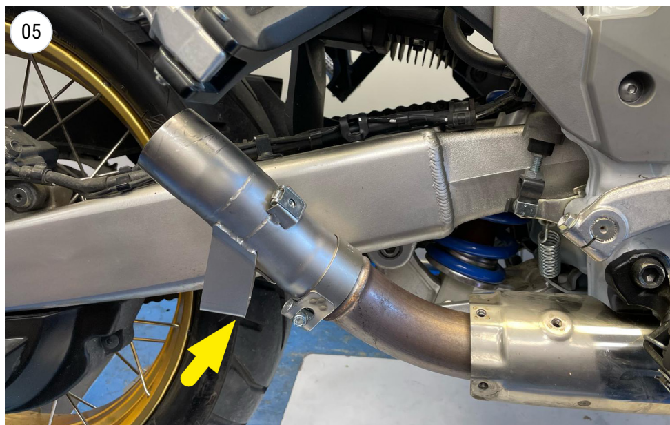
install the pipe with the clamp
