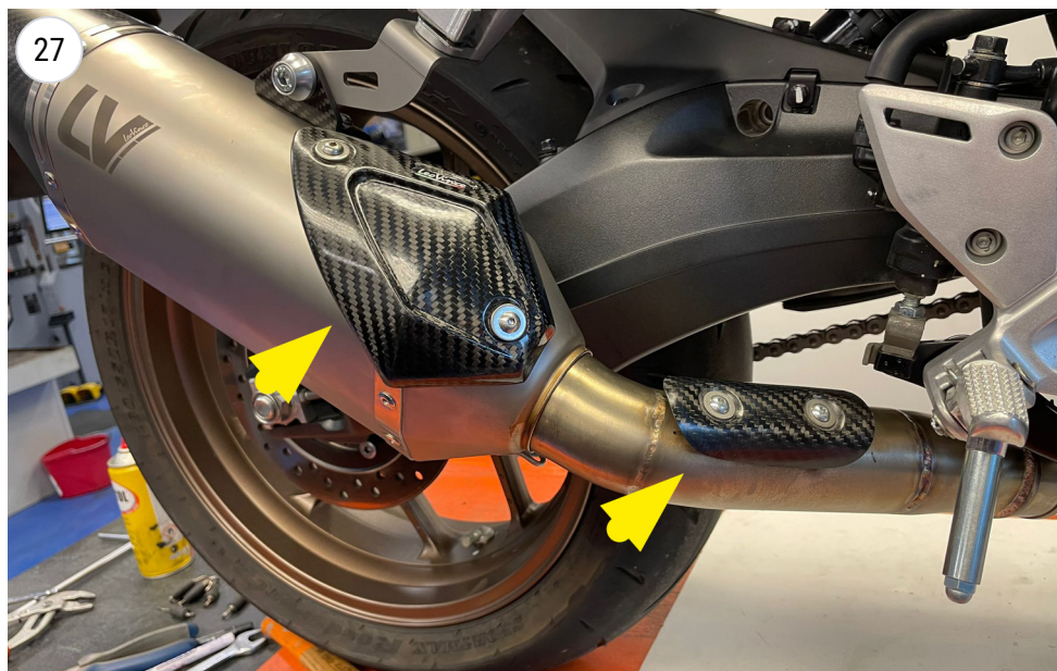
install the carbon heat shields
