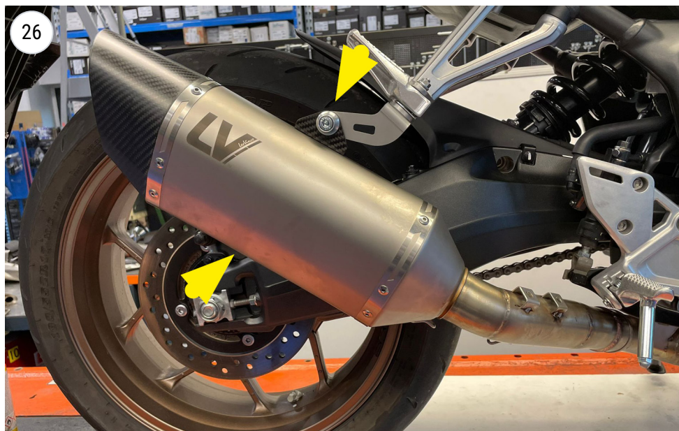
fit the muffler and screw
