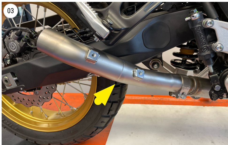
install the pipe
