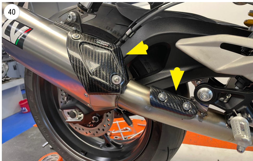
FIT THE CARBON HEAT SHIELDS
