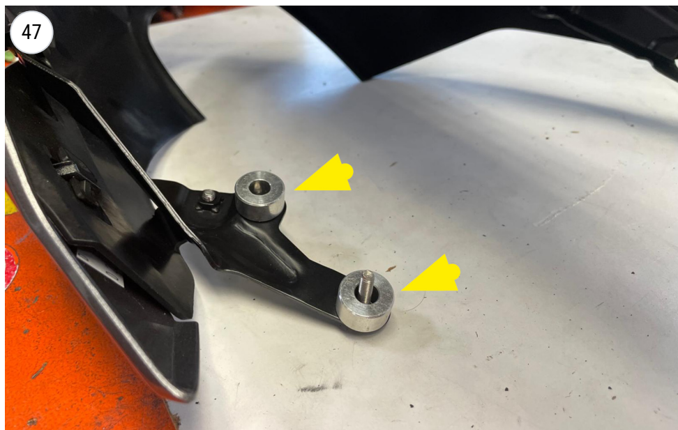
FIT THE SPACER ON THE LOWER FAIRING
