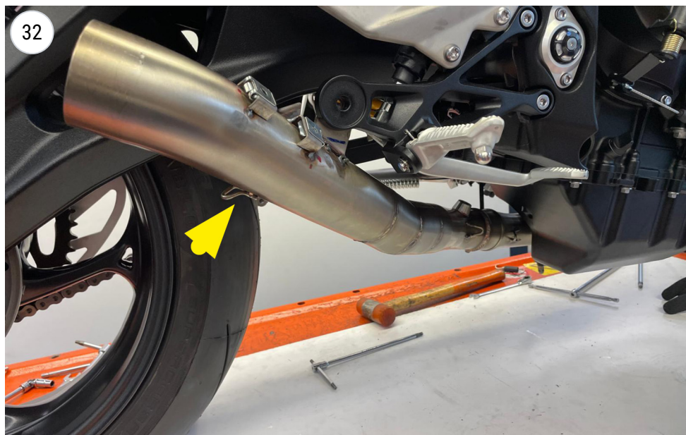
FIT THE FINAL LEOVINCE PIPE
