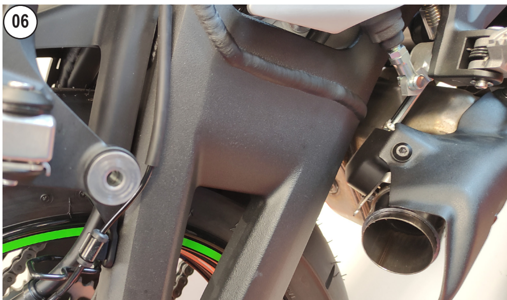
REMOVE THE FINAL PIPE
