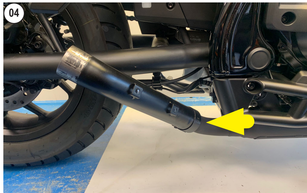
PUT THE LeoVince CLAMP ON THE LeoVince PIPE AND INSTALL IT
