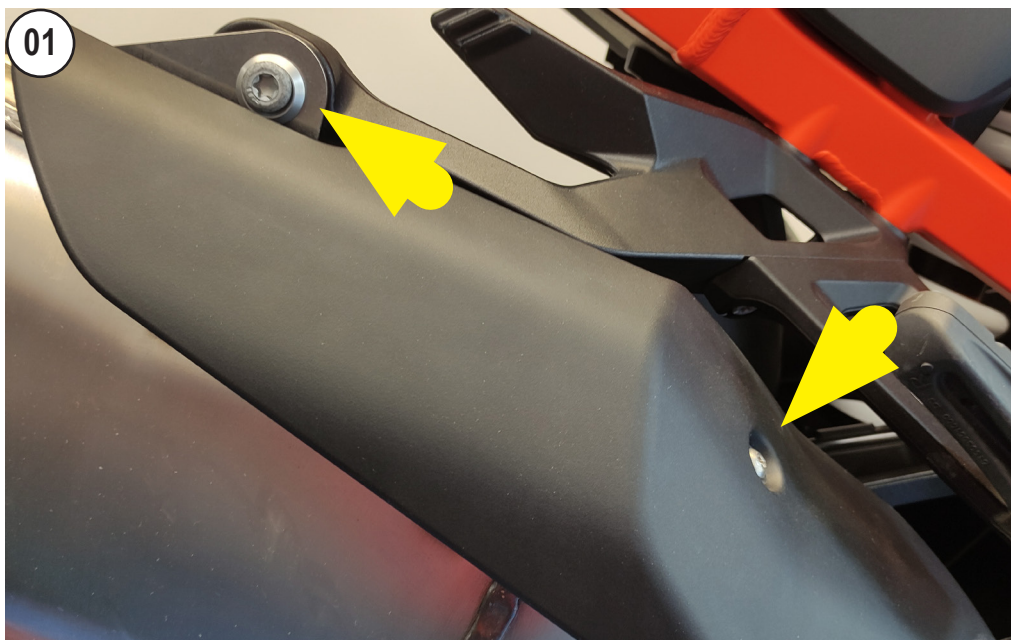
UNSCREW AND REMOVE THE HEAT SHIELD
