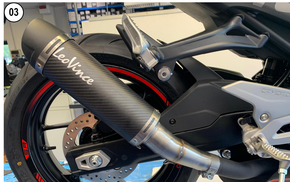
INSTALL THE MUFFLER
