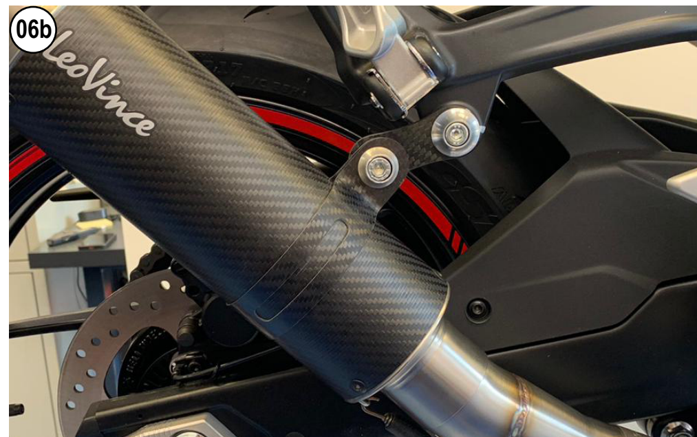
INSTALL THE CARBON CLAMP (ON GP CORSA MATTE)
