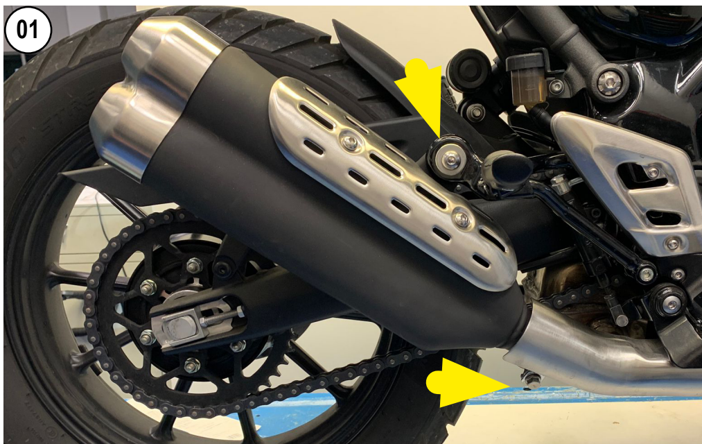
UNSCREW THE FASTENERS, LOOSE THE CLAMP AND REMOVE THE STOCK MUFFLER
