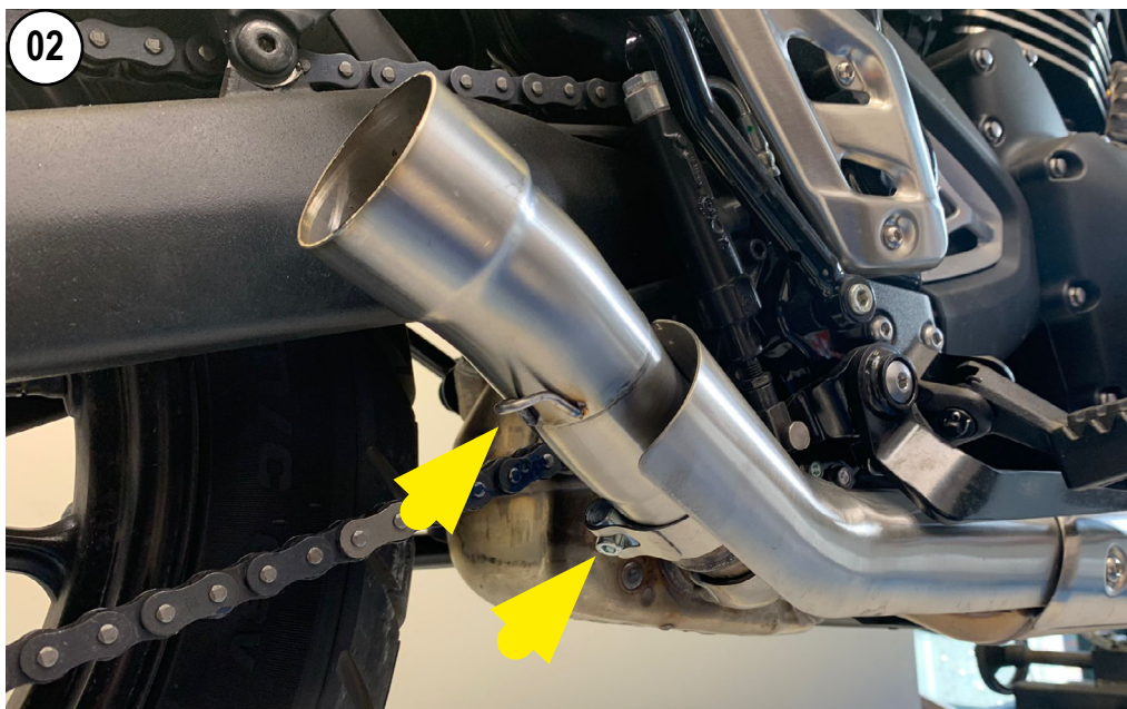
PUT THE S.S. CLAMP ON THE PIPE AND INSTALL THE PIPE
