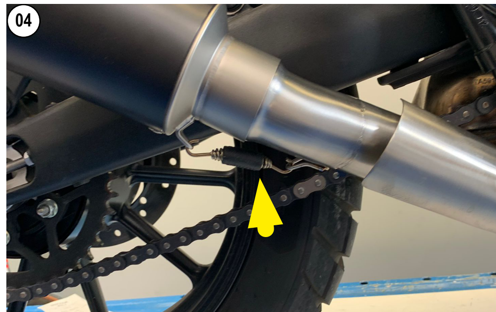
HANG THE SPRING AND TIGHTEN THE CLAMP
