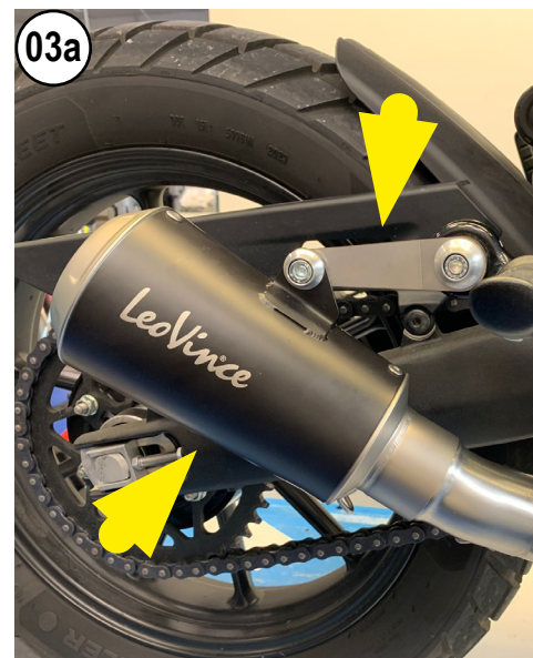
INSTALL THE MUFFLER, BRACKET AND FASTENERS
