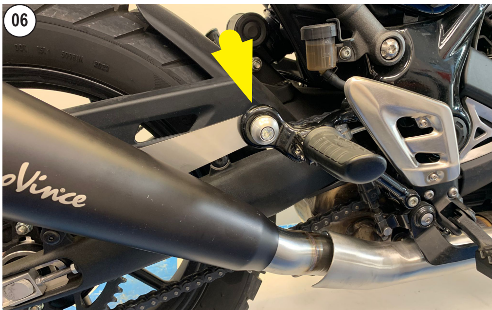
INSTALL THE MUFFLER, BRACKET AND FASTENERS
