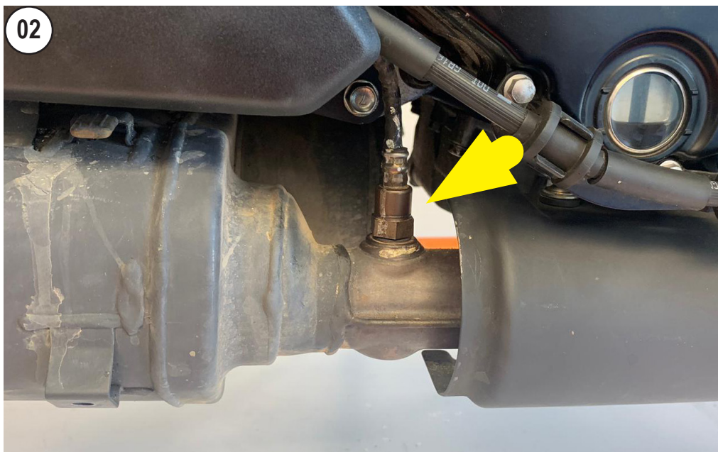
UNSCREW AND REMOVE THE LAMBDA SENSOR
