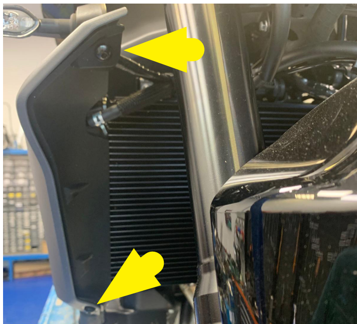
UNSCREW AND REMOVE THE FAIRING
