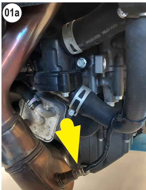
UNSCREW THE LAMBDA SENSOR
