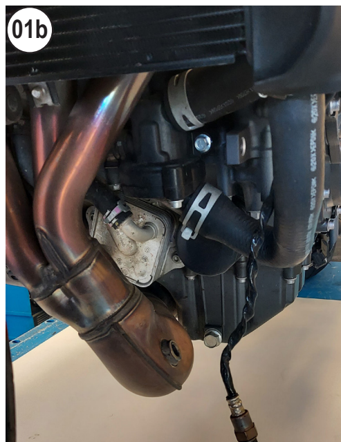
UNSCREW THE LAMBDA SENSOR
