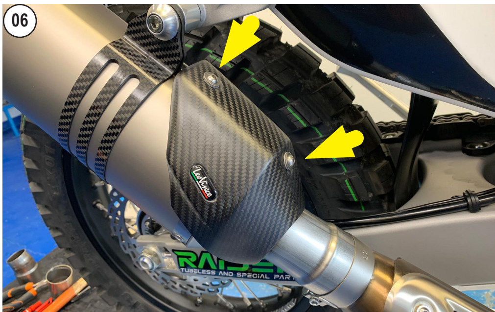
INSTALL THE CARBON HEAT SHIELD
