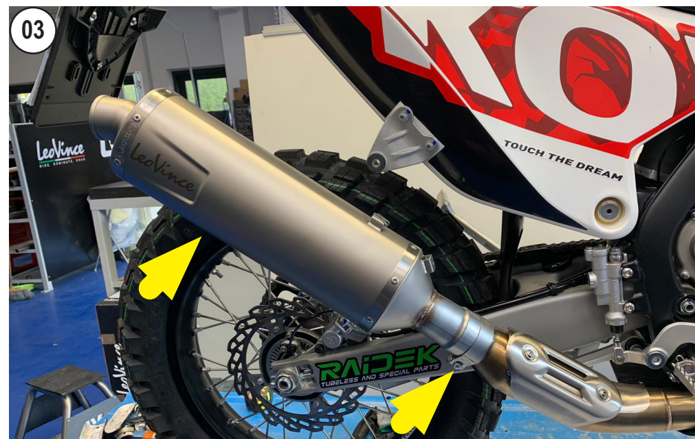
FIT THE CLAMP TO THE LEOVINCE PIPE AND INSTALL THE MUFFLER
