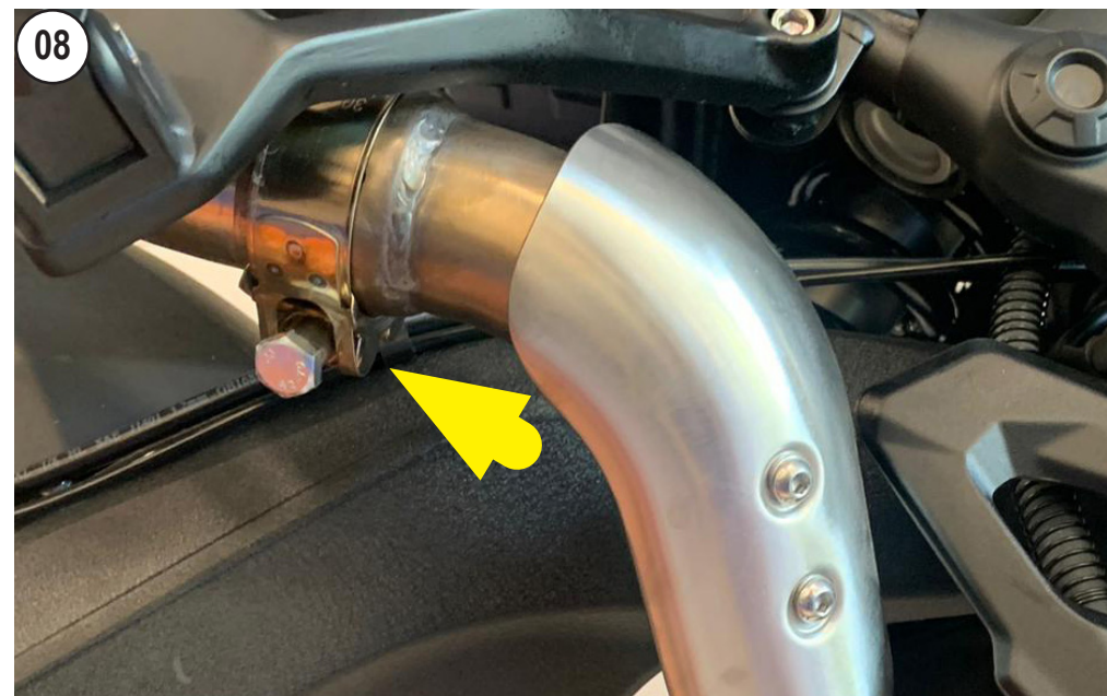
SCREW THE STOCK CLAMP
