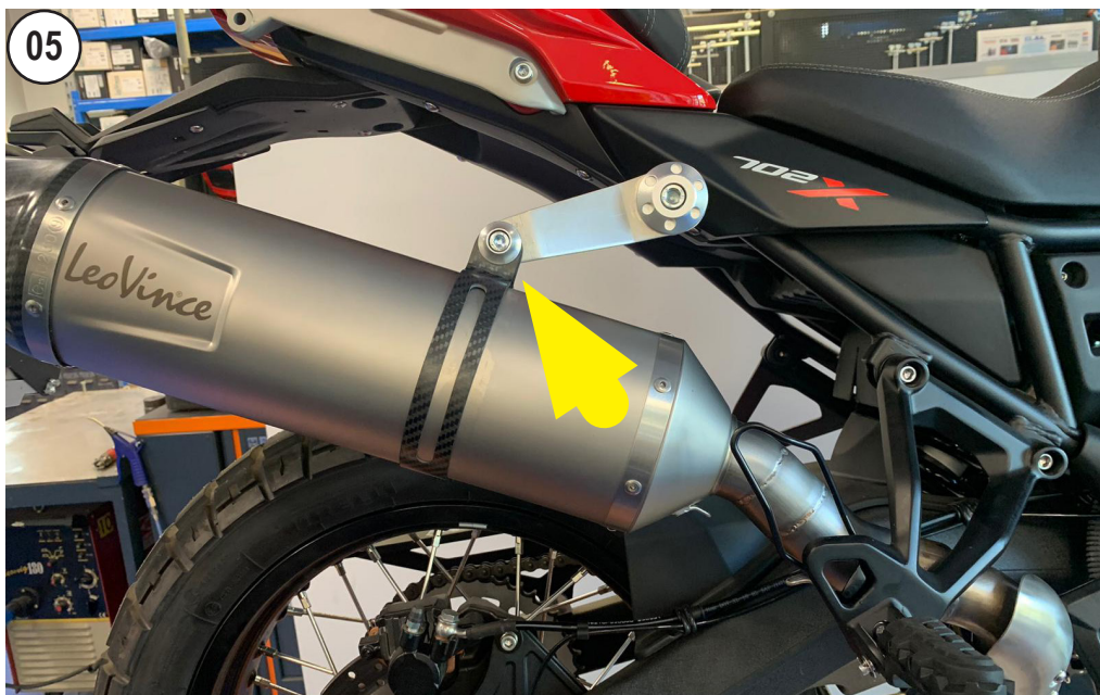
FIT THE LeoVince MUFFLER AND SCREW
