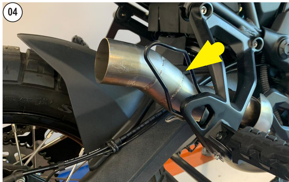
INSTALL THE LeoVince PIPE
