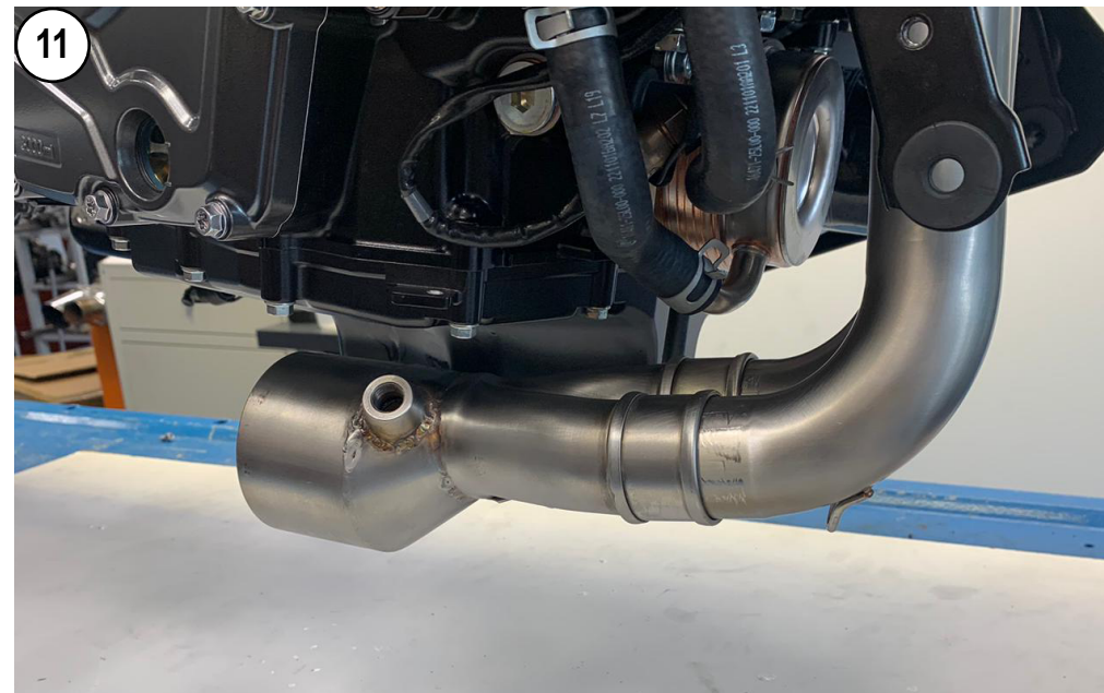
SLIDE IN THE SECONDARY PIPE
